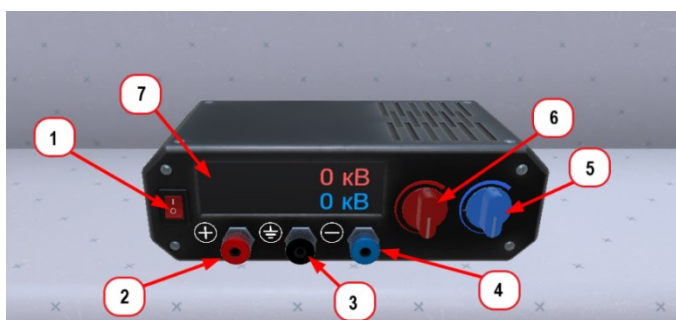
Figure 52 – High voltage source
