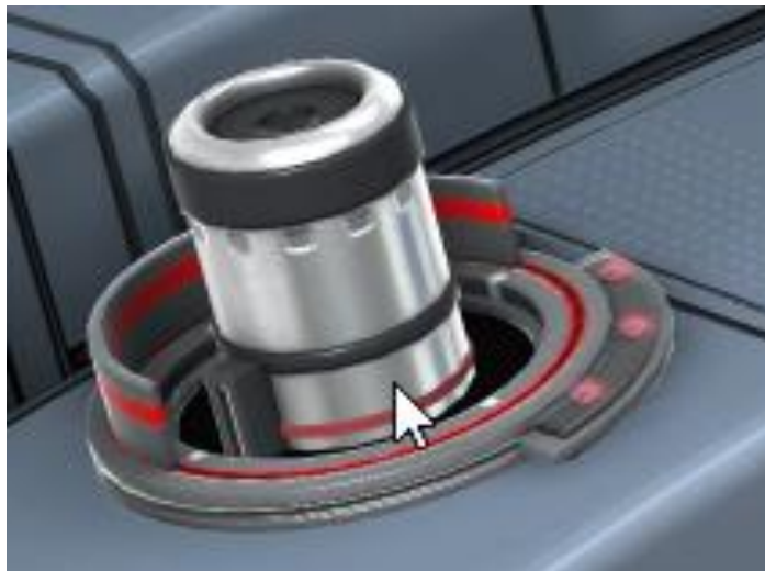
Figure 25 – Removing a gas lamp
