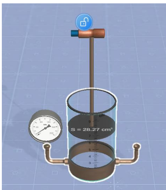
Figure 40 – Pressure gauge mounted on the piston container
