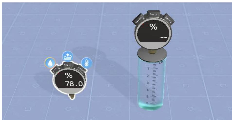
Figure 47 – Relative humidity readings on the universal meter
