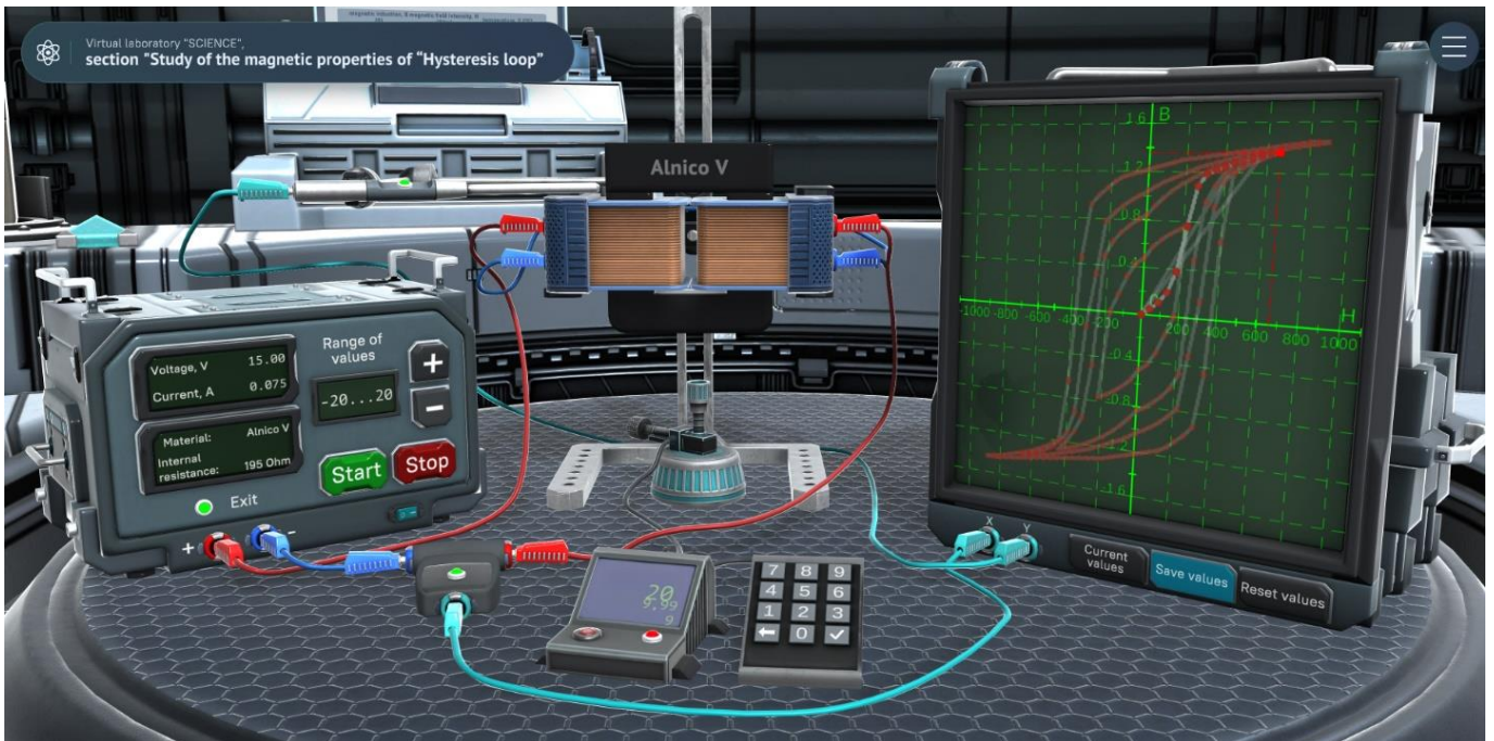
Figure 27 – Study of the hysteresis loop
