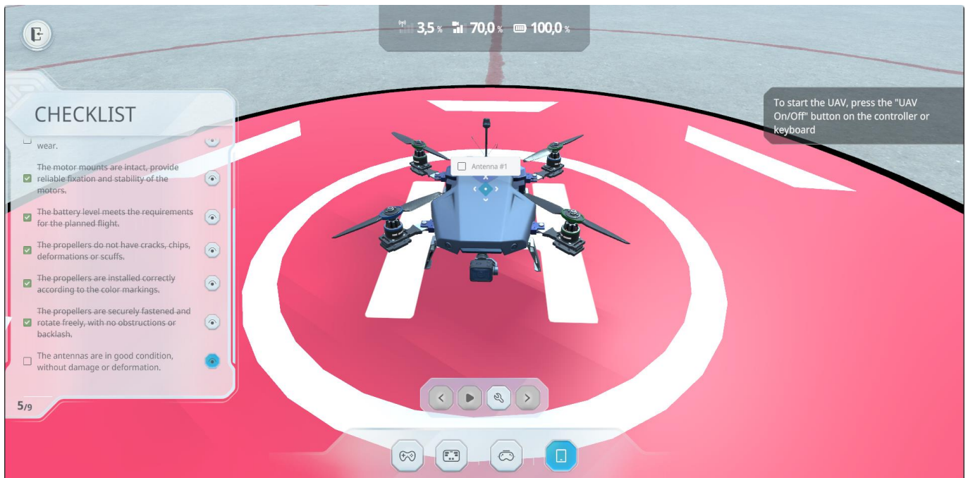
Figure 118 – Damaged part (antenna) detected
