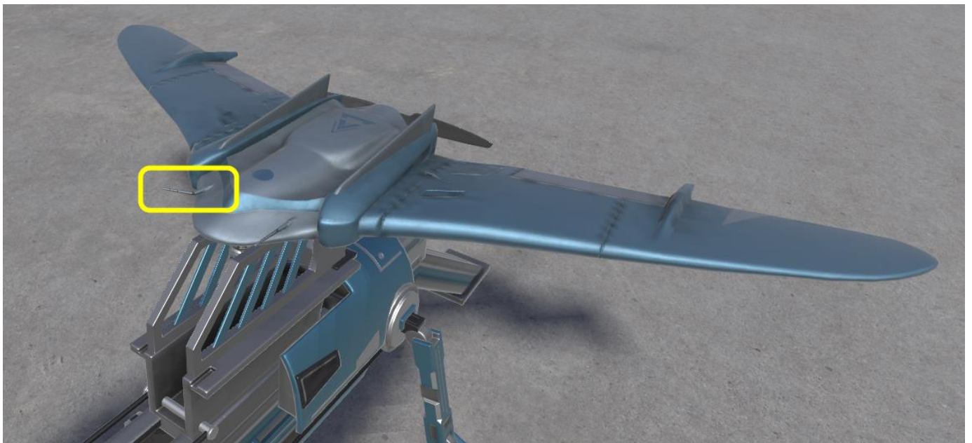
Figure 127 – Defect — antenna breakdown on an aircraft-type UAV
