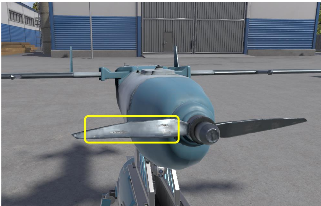
Figure 123 – Defect – chips on the propeller of an aircraft-type UAV
