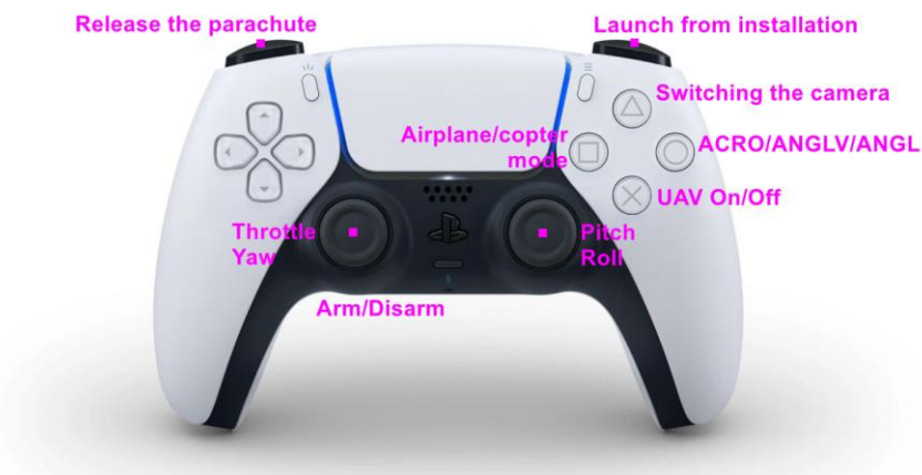
Figure 1 – PS controller controls
