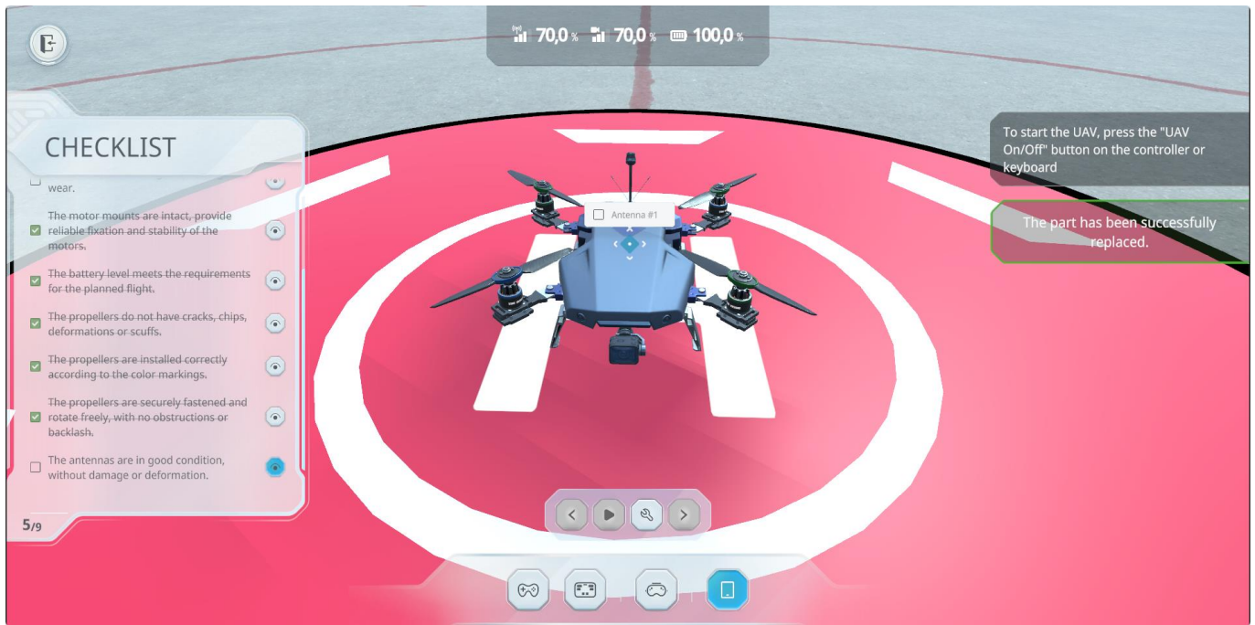
Figure 119 – The detected damaged part (antenna) is repaired
