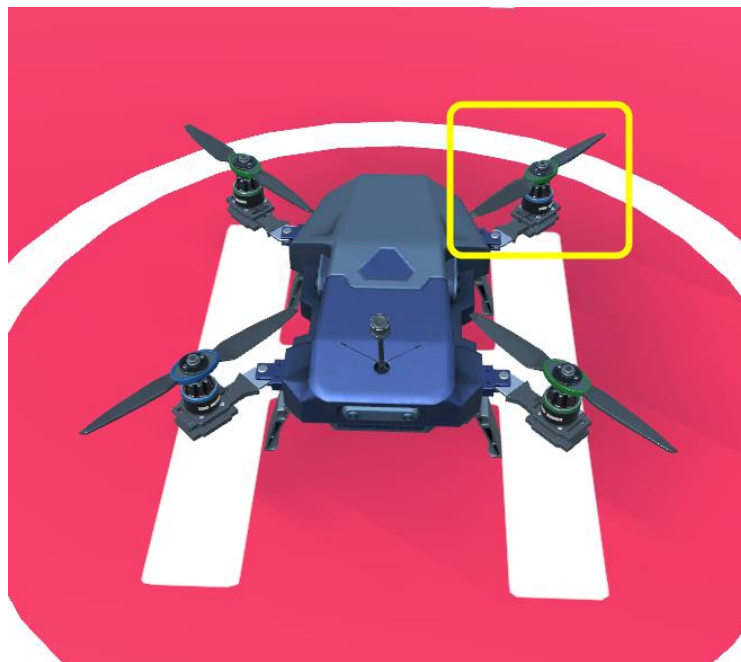
Figure 125 – Defect – incorrect installation of propellers
